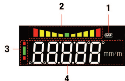
1. Battery status, 2. X-axis digital bubble 3. Y-axis digital bubble, 4. X-axis value
